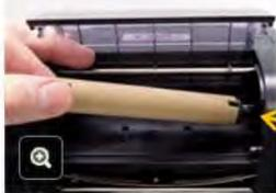
Take the empty spool removed in the previous step and install onto the ribbon rewind hub by pushing the spool against the hub spring and then positioning the spool onto the left hub.
