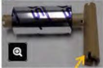
The old printer ribbon spool will be needed to collect the used ribbon from the new roll.
