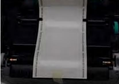
Once the media guides have been properly adjusted, the media must be positioned across the Media sensor and platen roller. Note that the left side of the media should be in alignment with the Media sensor. To verify alignment, carefully bend back the media strip and note the alignment of a black mark and the sensor. Pull the media strip across the Media sensor and platen roller. The tape strip can be used to temporarily hold the media strip in place while closing the top cover.
