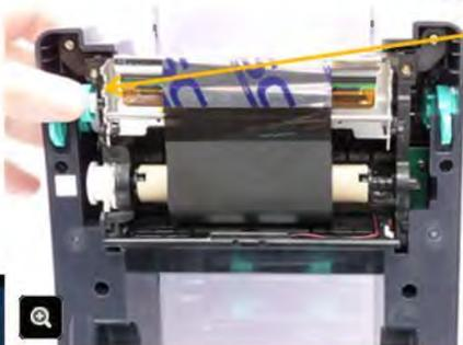
**Turn the ribbon rewind gear until the ribbon leader is completely wound onto the rewind spool and the black section of the ribbon covers the print head.**
