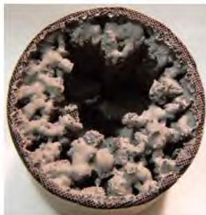
TWC internal damage as shown in the photograph, is caused by excessive heat resulting from excessive amounts of unburned fuel passing through the engine. As the unburned fuel (HCs) come in contact with the catalyst sites, the hydrogen and carbon atoms separate, releasing a large amount of heat energy. If too much heat energy is released in a short amount of time, the metal and ceramic materials will melt.
