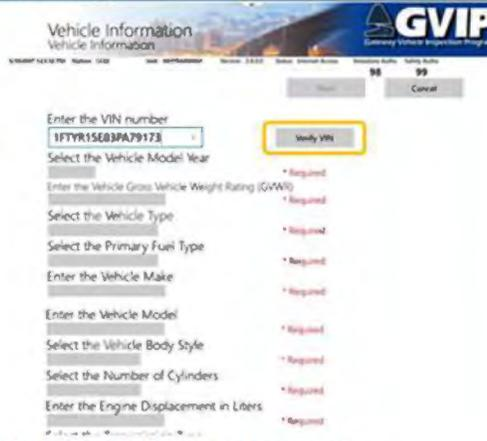
To begin, enter the VIN of the vehicle being tested using the tablet's built-in bar code scanner (described in Section 2) or using the keyboard to manually input the VIN. When entered correctly, a VIN for a 1996 and newer vehicle will have 17 characters. Once the VIN has been entered, select the Verify VIN button.
