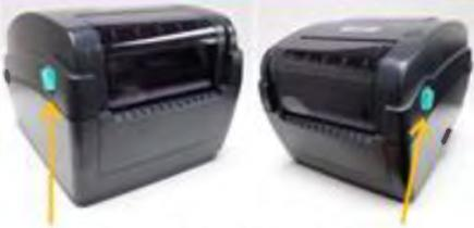
In order to open the sticker printer top cover, both the left and right top cover open levers must be moved forward simultaneously.
