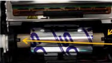
Install the new printer ribbon roll onto the right supply hub, paying attention to align the slots in the spool with the hub splines, and then mount the spool on to the left hub with spool slots aligned with hub splines.
