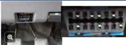
All 1996 and newer light-duty vehicles with spark-ignition engines and all 1997 and newer light-duty vehicles with compression-ignition engines have the required DLC.
