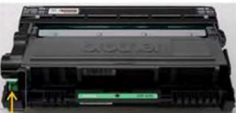
To release the toner cartridge from the drum unit, press down on the lock lever as described in the instructions. (Click the lever in the picture to get an idea of how much toner cartridge movement to expect. Click here to reset image.)
