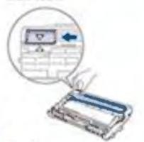
10. Push the tab to return the tab to the Home position (H). This arrow on the tab must be aligned with the arrow on the drum unit. If it is not, printed pages may have a vertical edge.
